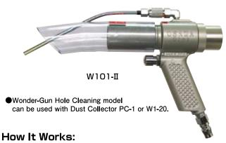
Put Air Blow Nozzle into a hole and then press Air Valve. Air comes out from the nozzle, and blow dust off. The dust is cleaned by the Transparent pipe.
