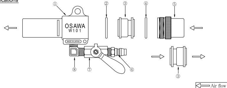
③To change the direction of air flow, just reposition the suction nozzle. Please confirm the direction before operation.
