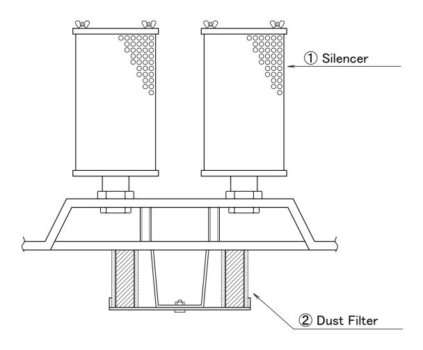
Please use the fine dust filter set for collecting fine dust/ powders, as this model is not designed for fine dust collection.
