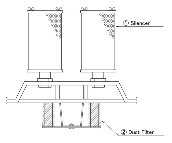
Please use the fine dust filter set for collecting fine dust/ powders, as this model is not designed for fine dust collection. To order the filter set, please specify as FINE DUST FILTER SET (Large), available from 1 set.
