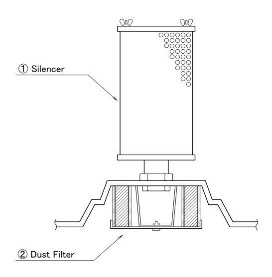
Please use the fine dust filter set for collecting fine dust/ powders, as this model is not designed for fine dust collection. To order the filter set, please specify as FINE DUST FILTER SET (Large), available from 1 set.
