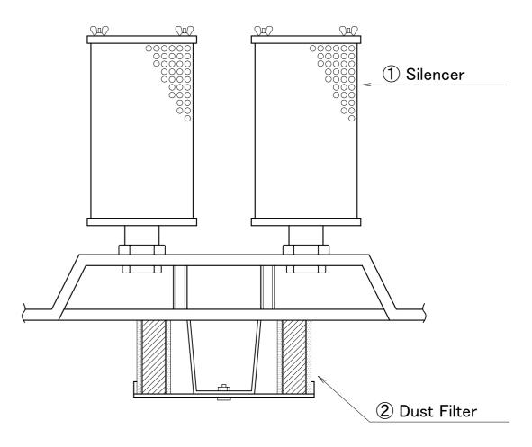
Please use the fine dust filter set for collecting fine dust/ powders, as this model is not designed for fine dust collection.
