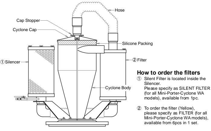
Frequent maintenance is not needed for Mini-Porter-Cyclone. However, occasional cleaning is required in the inside of the body to maintain optimal performance. To clean, brush the inside occasionally. Especially after vacuuming the moist dust, brush well or wipe well with the dry cloth since the moist dust stays inside.
