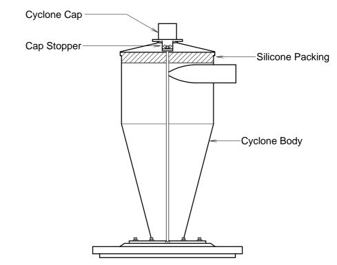
X Frequent maintenance is not needed for Mini-Porter-Cyclone. However, occasional cleaning is required in the inside of the body to maintain optimal performance. To clean, brush the inside occasionally. Especially after vacuuming the moist dust, brush well or wipe well with the dry cloth since the moist dust stays inside.
