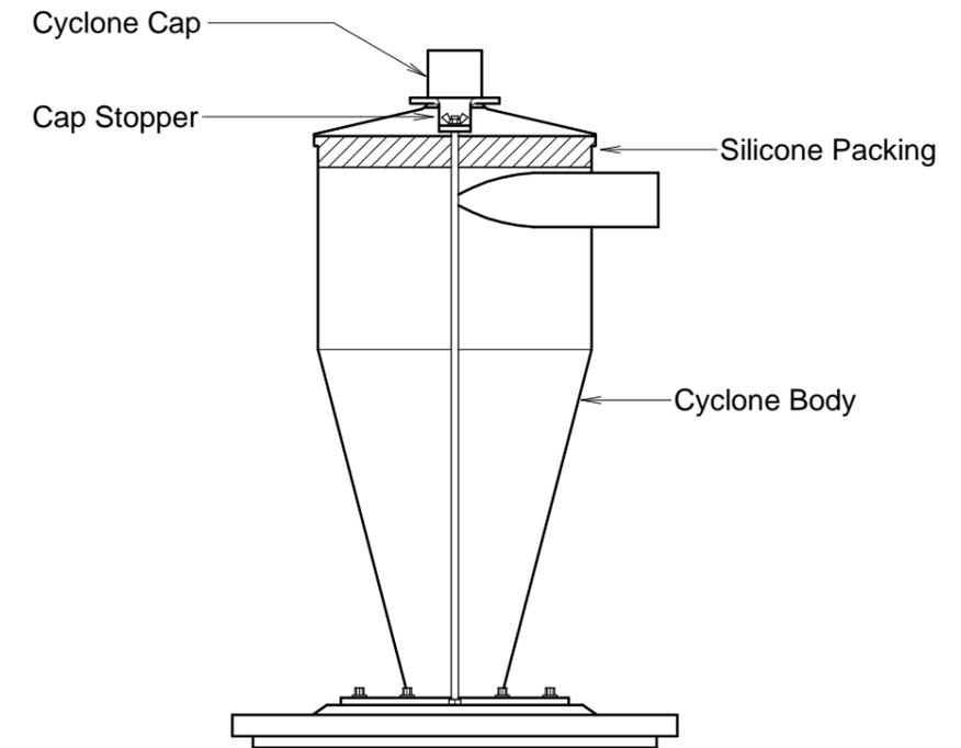
※ Frequent maintenance is not needed for Mini-Porter-Cyclone. However, occasional cleaning is required in the inside of the body to maintain optimal performance. To clean, brush the inside occasionally. Especially after vacuuming the moist dust, brush well or wipe well with the dry cloth since the moist dust stays inside.
