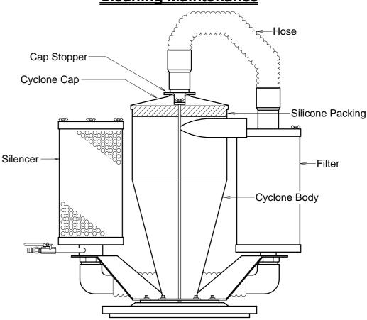
※ Frequent maintenance is not needed for Mini-Porter-Cyclone. However, occasional cleaning is required in the inside of the body to maintain optimal performance. To clean, brush the inside occasionally. Especially after vacuuming the moist dust, brush well or wipe well with the dry cloth since the moist dust stays inside.
