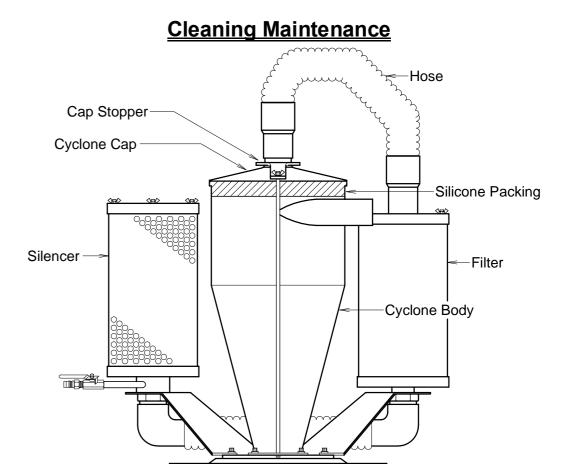
Frequent maintenance is not needed for Mini-Porter-Cyclone. However, occasional cleaning is required in he inside of the body to maintain optimal performance. To clean, brush the inside occasionally. Especially after vacuuming the moist dust, brush well or wipe well with the dry cloth since the moist dust stays inside.
