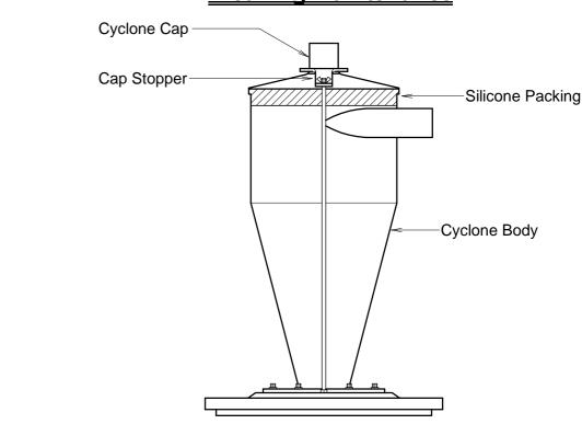
the inside of the body to maintain optimal performance. To clean, brush the inside occasionally. Especially after vacuuming the moist dust, brush well or wipe well with the dry cloth since the moist dust stays inside.
