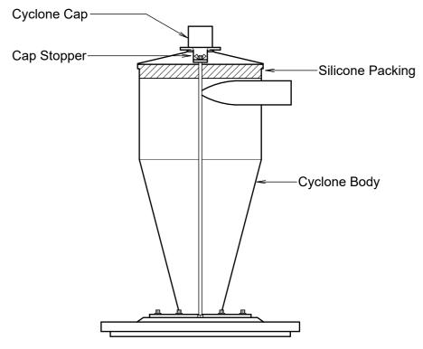
※ Frequent maintenance is not needed for Mini-Porter-Cyclone. However, occasional cleaning is required in the inside of the body to maintain optimal performance. To clean, brush the inside occasionally. Especially after vacuuming the moist dust, brush well or wipe well with the dry cloth since the moist dust stays inside.
